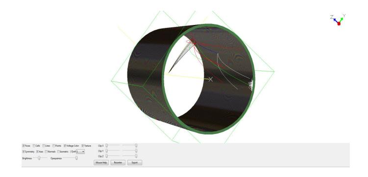
Cylinder pore model with potential gradient defined (can be scaled) Validation of the secondary emission model SIMION smooths adjacent grids in this geometry.
