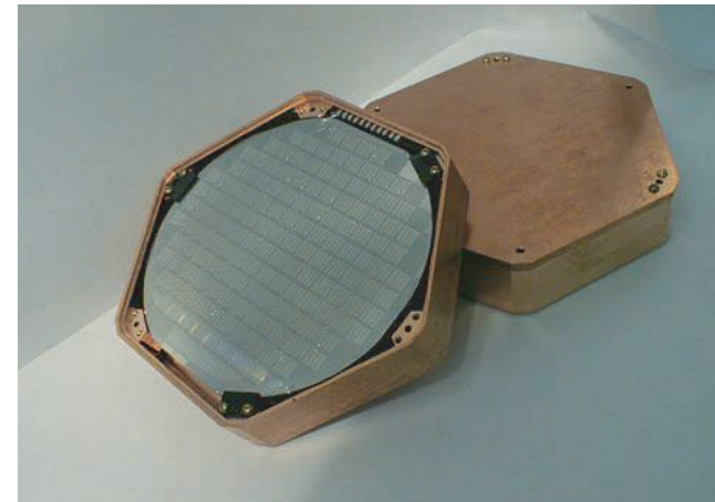
Germanium detector (as in CDMS, Edelweiss)
