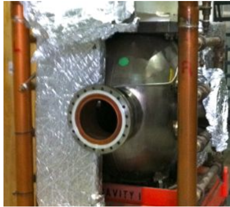
Fig. F.1. One of two 500 MHz room-temperature RF cavities arrived from Daresbury
