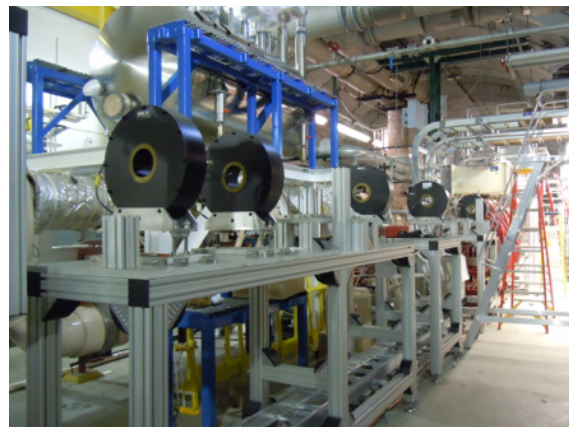
Fig. H.7. Left: The CeC's quiet helium source (top-right) is installed at IP2 above RHIC magnets. The photo was taken when the first of two LiHe transfer lines to 113 MHz gun is being installed. Right: The solenoids on their supports installed in the IP2.
