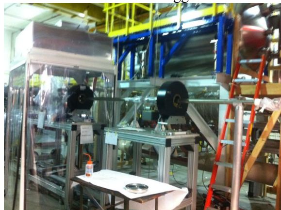
Fig. H.8. Left: Phase I (low energy) beamline with solenoids (black) and vacuum pipes during installation; Right: Water-cooling distribution system for 500 MHz (seen on the background) and 113 MHz system
