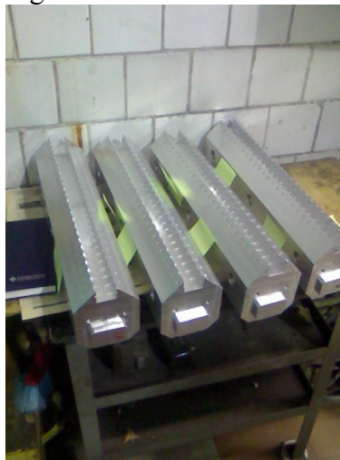
Fig. F.2. Four magnet holders for the wiggler at BINP's workshop.
