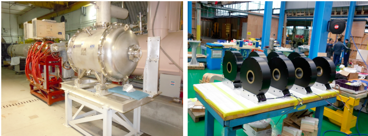
Fig. H.6. Left: The 113 MHz SRF gun and the 500 MHz RF cavities at 2 o'clock RHIC IP. Right: The CeC solenoids at the vendor facility
