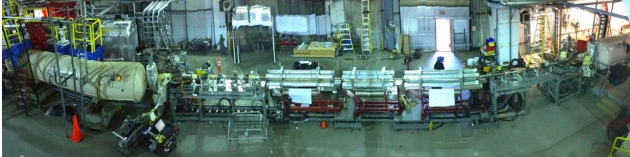
Fig. H.16. Installed CeC section with three-wiggler FEL– common with RHIC
