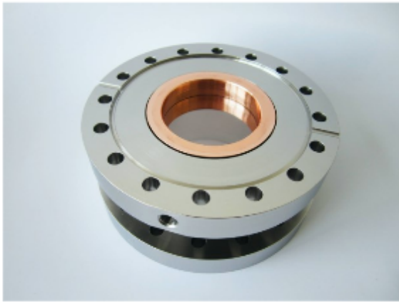
Fig. H.22. Left: SVD diamond window; Right: retuning of the SRF gun frequency to a harmonic of 2.6.5 GeV/u Au ions revolution frequency
