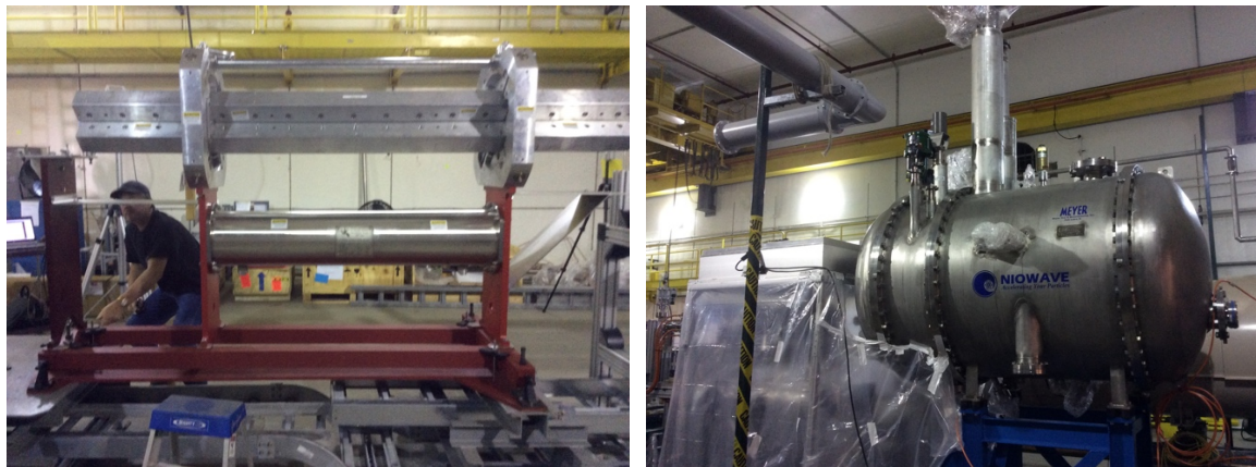
Fig. H.14 Left: The first helical wiggler installed in the RHIC tunnel; Left: 704 MHz SRF linac cryomodule arrived to BNL and moved to IP2
