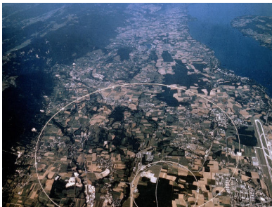
The 27km LEP ring was reused to build the Large Hadron Collider
