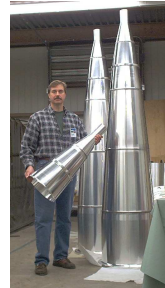
NuMI Horn 2 inner conductor Radial field, B \propto 1/r
