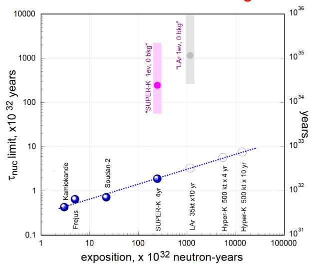
24 candidate events in Super-K might contain several genuine n-nbar events. Backgroundless detectors needed to explore nnbar > 10<sup>33</sup> years. Can atmospheric neutrinos and nnbar signals be separated in LAr detectors? 33
