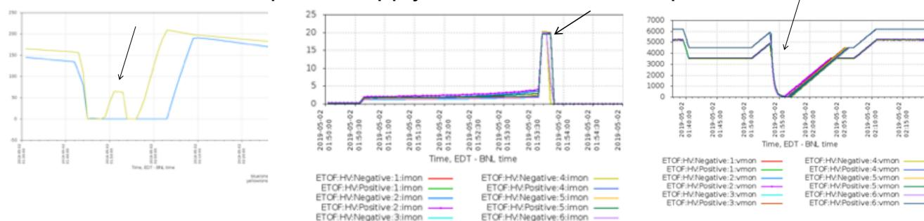
Hypothesis: beam loss events → high flux of particles → induced high current in very short time in readout electrodes → damaged PADI input stage
