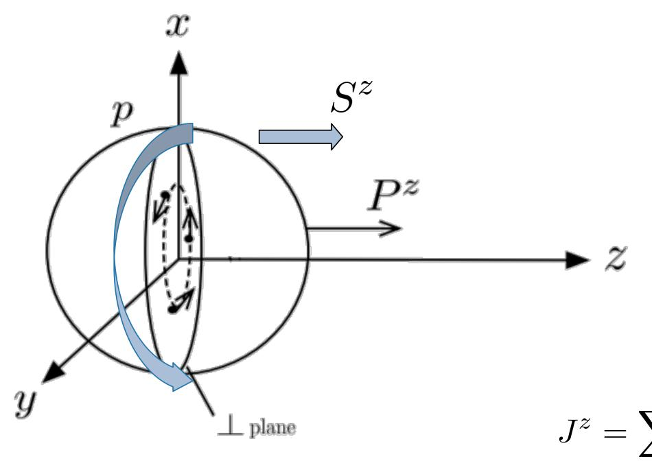
$$J^z = \sum_i r_i^x p_i^y - r_i^y p_i^x$$
