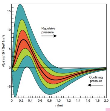
Pressure distribution obtained from fits to Jlab data to extract the GPDs, in particular the D-term
