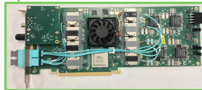
TPC FEE, 160k ch BNL-712 / FELIX v2 x48 (ATLAS/sPHENIX) SAMPA (ALICE/sPHENIX)
