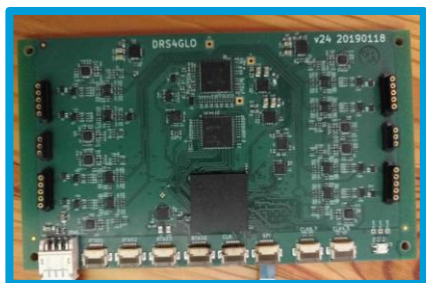
Precision timing digitizer DRS4GIO (SBIR/LDRD)
