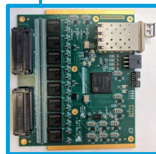
TPC FEE, 160k ch BNL-712 / FELIX v2 x48 (ATLAS/sPHENIX) SAMPA (ALICE/sPHENIX)
