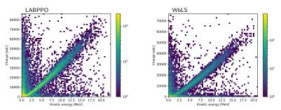
Bin in neutron energy and fit with Gaussian + exponential
