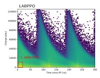
Fit to timing of  $\gamma$  sample yields gross time-of-flight calibration and beam profile
