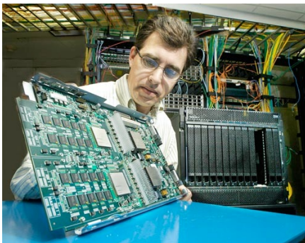
blade11bc4 @IBM, Böblingen: 2 Cell Broadband Engines, 256 kB LS, 2.4 GHz
