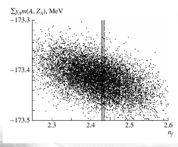
**Fig. 2.** Effect of the errors in the yield of products originating from <sup>235</sup>U fission on the mass defect  $\sum y_A m(A, Z_A)$  (see main body of the text). The vertical band corresponds to the experimental value of the number  $n_f$  of neutrons.
