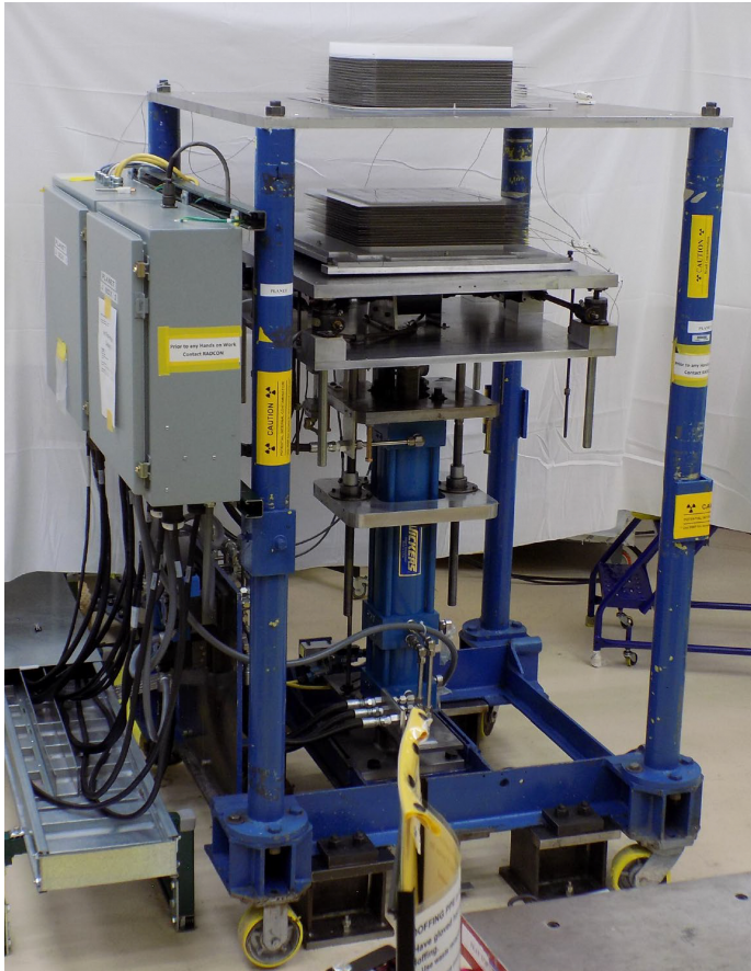
Picture of TEX-Pu Configuration on Planet Vertical Lift Machine at the National Criticality Experiments Research Center (NCERC), Photo credit Los Alamos National Laboratory
