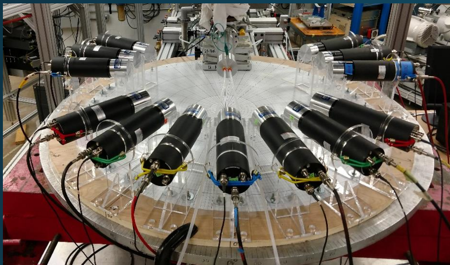
2018, Secondary \gamma -ray angular distribution setup with HAGRID
