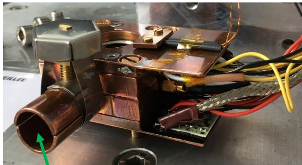
Cold finger for liquid nitrogen
