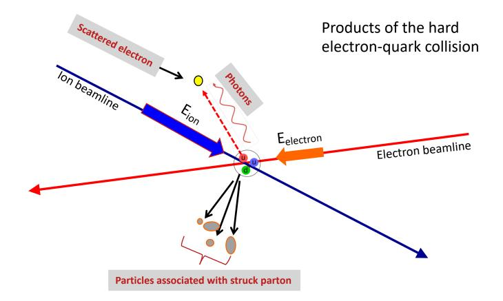
Asymmetric collision energies will boost the final state particles in the ion beam direction: **Detector requirements change as a function of rapidity.**
