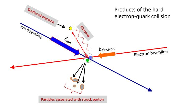
**Transverse and flavor structure measurement of the nucleon and nuclei**: The particles associated with struck parton must have its species identified and measured. **Particle ID much more important than at HERA** colliders.
