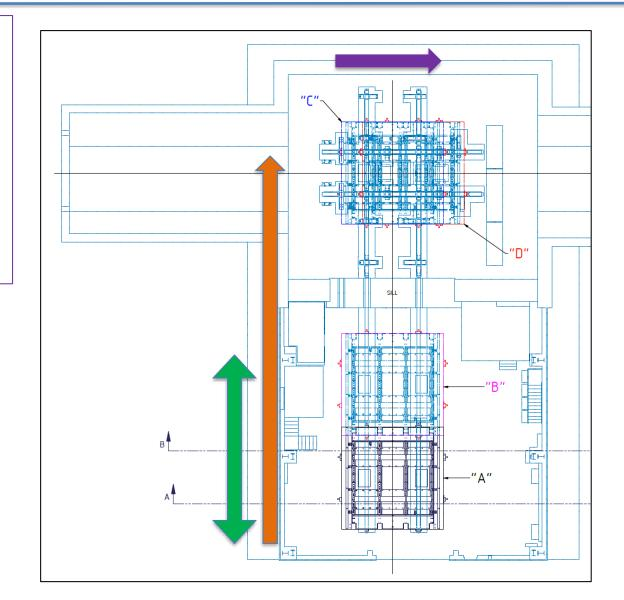
Access to the Babar magnet stabilizing tension rods is lost once the Inner Support Rings are installed
