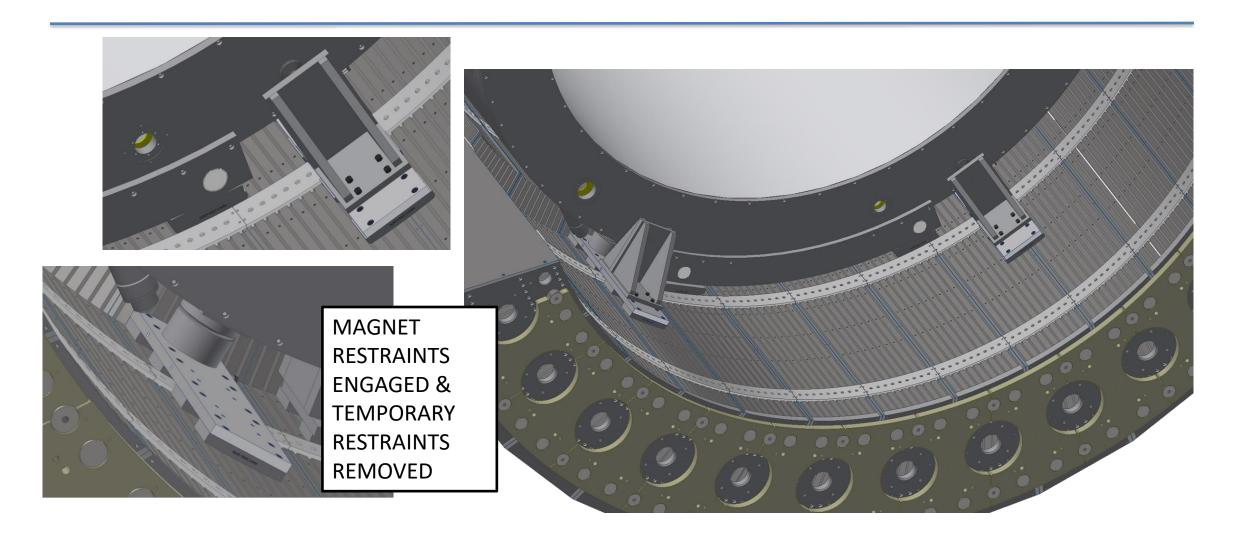
Step #3: Lower magnet in to position on lower pads and locating features
