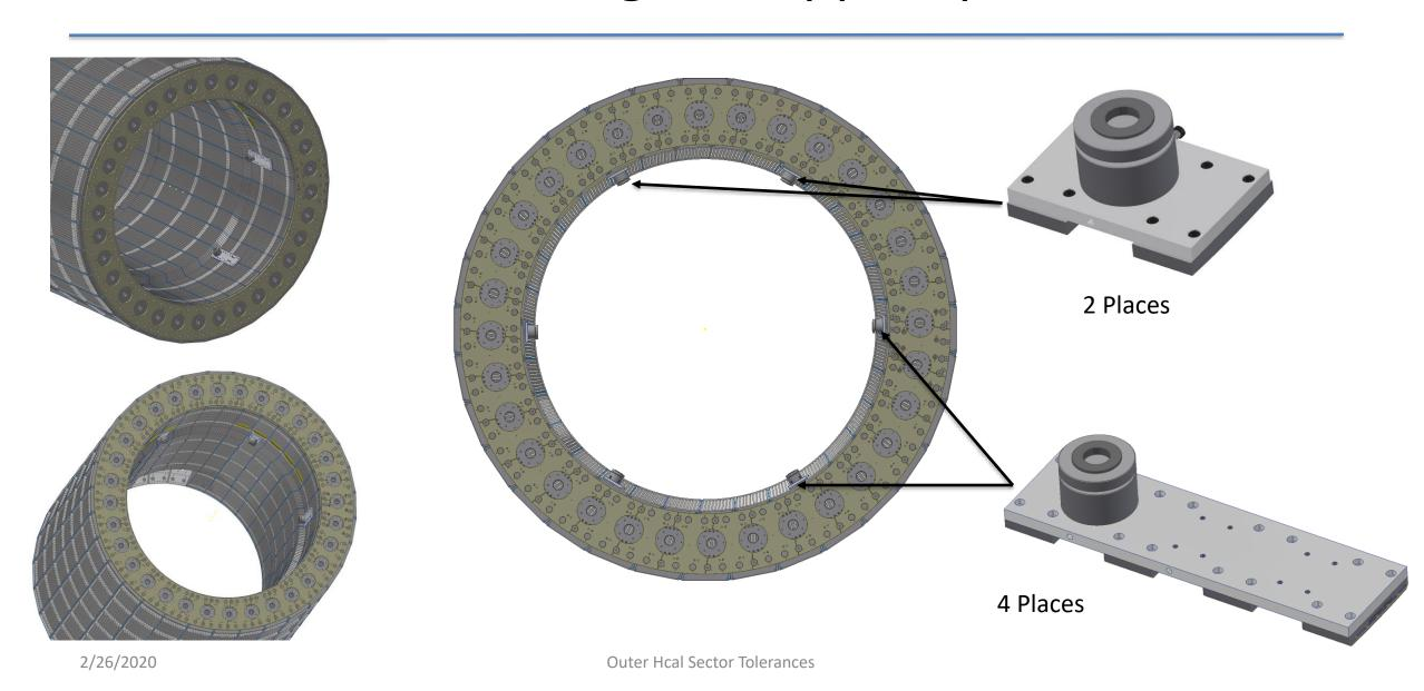
Step #2: Magnet locating and support feature attached to cryostat
