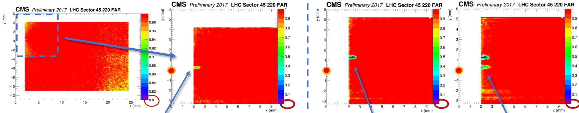
Lower efficiency caused by the radiation damage
