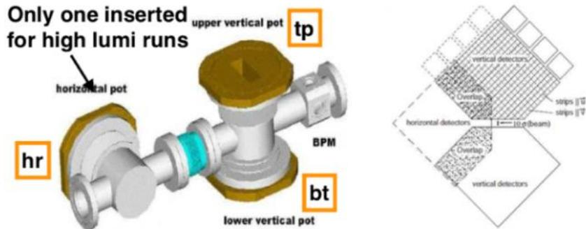
Tracking RPs **equipped with a thin window 150  $\mu\text{m}$  thick towards the beam**
