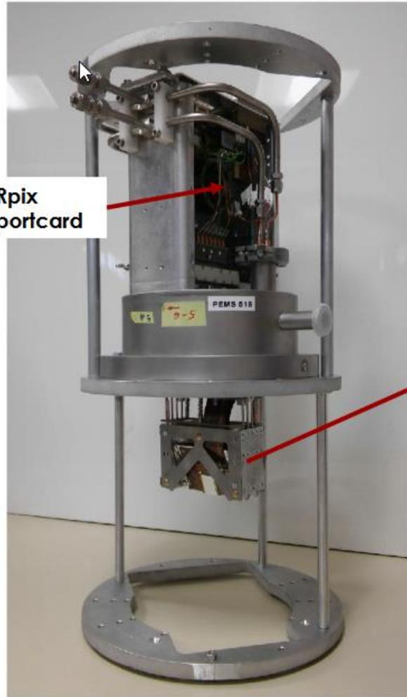
Each station contains **6 detector modules**, tilted by  $18.6^\circ$  to improve resolution
