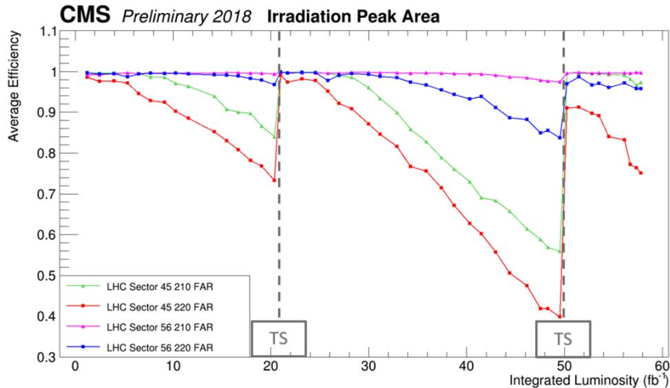
**Average efficiency** calculated every  $\sim 1 \text{ fb}^{-1}$  in the critical region (irradiation peak area)
