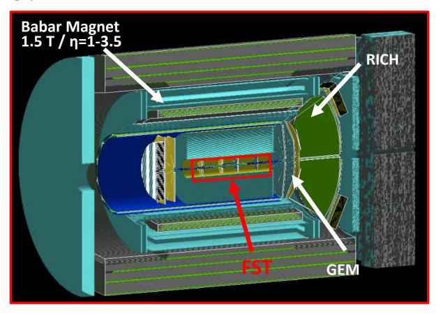
• Implement the LANL Forward Silicon Tracking detector (FST) with 6 forward planes in the forward region.
