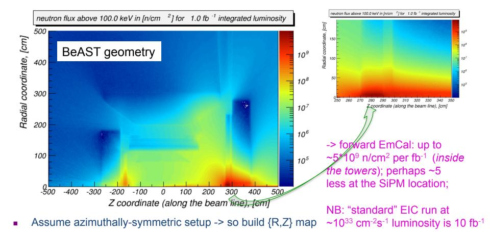
► Close to beam line: ~10<sup>34</sup> cm<sup>-2</sup>s<sup>-1</sup> over ~10 years would exceed ~10<sup>11</sup> n/cm<sup>2</sup>
