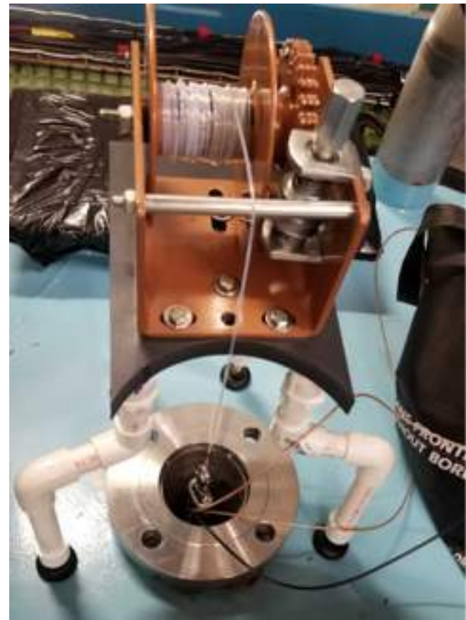
AmBe source deployment into ANNIE tank
