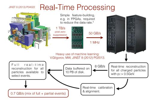
\*LHCb will move to a triggerless-readout system for LHC Run 3 (2021-2023), and process 5 TB/s in real time on the CPU farm.
