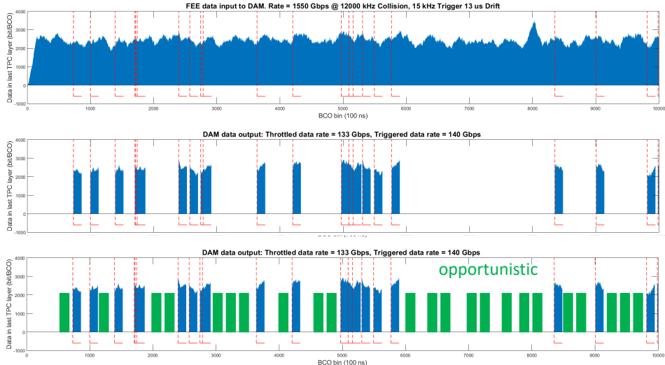
Figure 2: A simulation of the TPC data stream. The upper figure shows the continuously streaming data as a function of time, expressed as the beam crossing count (BCO). The dashed red lines denote accepted triggers. The lower figure shows the portion of the streaming data correlated with the accepted triggers. Each of the short blue sections in the lower figure is at least 13 \mu\text{s} long. The 4 th and 5 th trigger around BCO 1800 “extend” the TPC readout period, as do the triggers around BCO 2800 and 5000. The lower figure shows conceptually how we can “back-fill” free capacity by accepting additional tracking system-only events.
