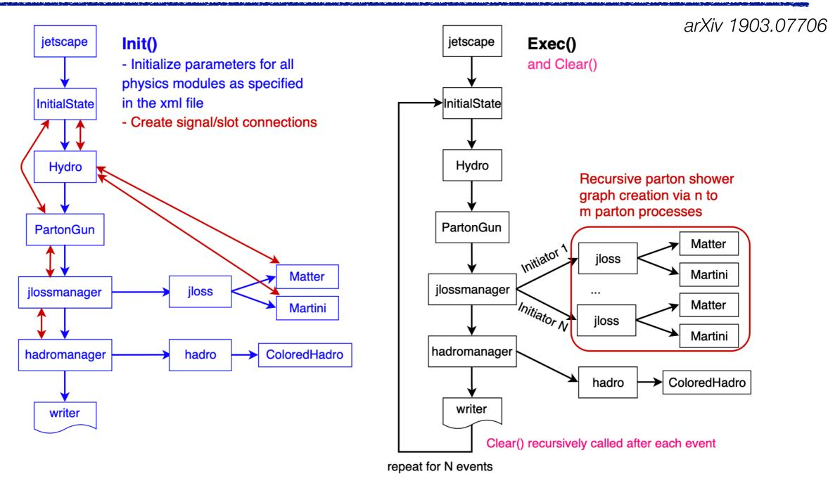
Figure 4: Example workflow of the Init() (left side) and Exec() (and Clear()) (right side) phase of the task based JETSCAPE framework (the not extensively used Finish() phase is omitted). One should be aware that the created signal/slot connections in the Init() phase are of course present and utilized in the Exec() phase, but are not show in the figure for simplicity.
