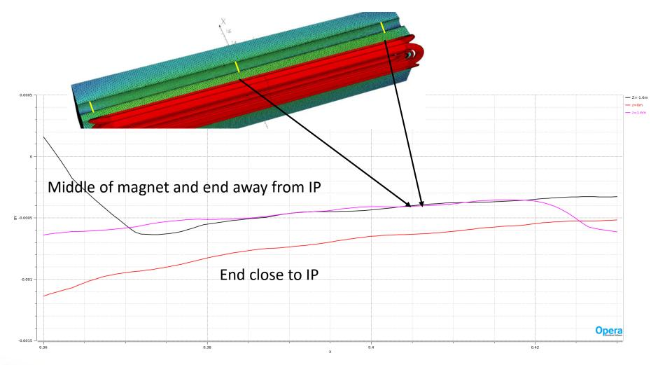
About 1 mT for end closer to IP Can be shielded with mu-metal
