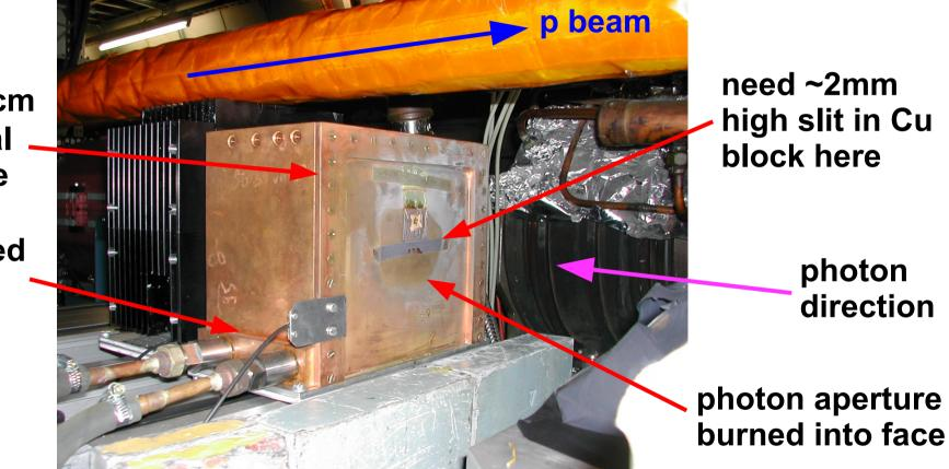
Similar design w/ water cooling (sync. rad.) may be adequate only in beam few minutes, not as severe as γ exit window/converter
