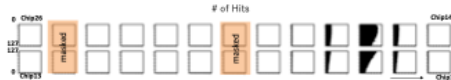
Hit distribution with scintillator as a quenching material.
