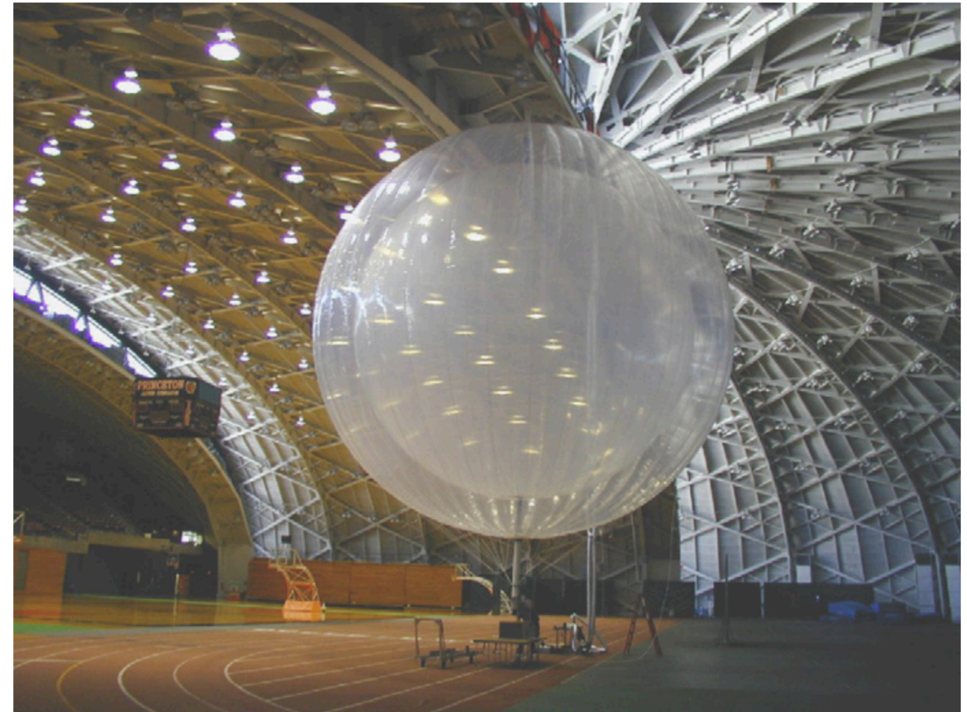
The nylon scintillator containment vessels for the Borexino solar neutrino experiment, J. Benziger et al. NIM, 2007
