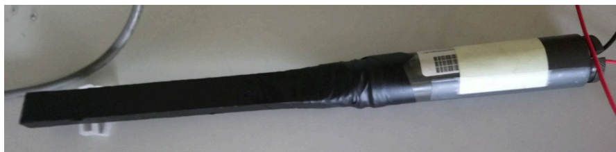
Scintillator size : 235 * 23.5 * 13 mm
