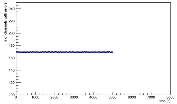
Number of APVs and channels with errors vs time.
