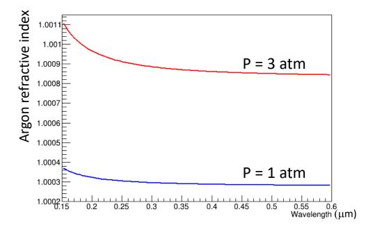
Argon refractive index vs wavelength (at atmospheric pressure)
