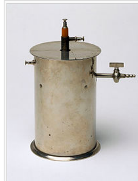
Ionization chamber made by Pierre Curie, c 1895-1900
