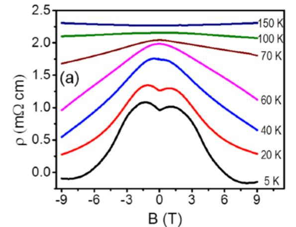
*measurement of conductivity in Weyl semimetal, from 1412.6543*
