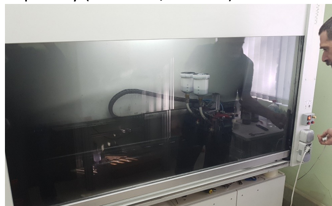
Automatic painting of the conductive layer on the glass
