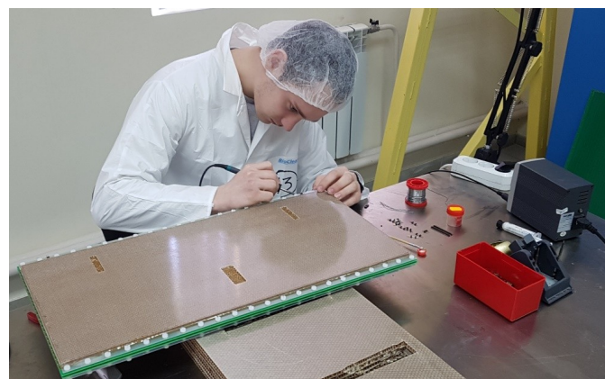
Soldering HV connector and readout pins
