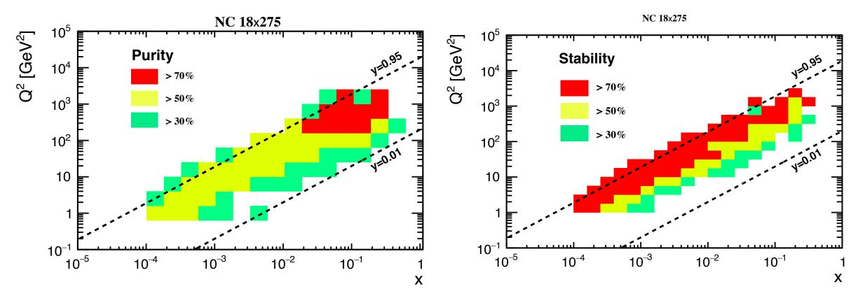
Note: The lack of coverage at low inelasticity is highlighted here. This region is filled in by the JB reconstruction and demonstrates what would be lost without forward coverage with good calorimeter and tracking resolution.
