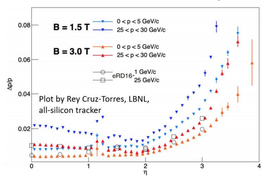
Realistic simulations show tracking performance deteriorates fast beyond eta = 3.0, but currently the detector matrix states:
