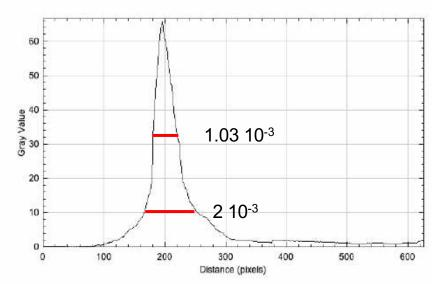
Scaling: 31 pixels per 1 mm, FWHM energy spread is 1.03 10<sup>-3</sup>; RMS energy spread is 4.4 10<sup>-4</sup>
