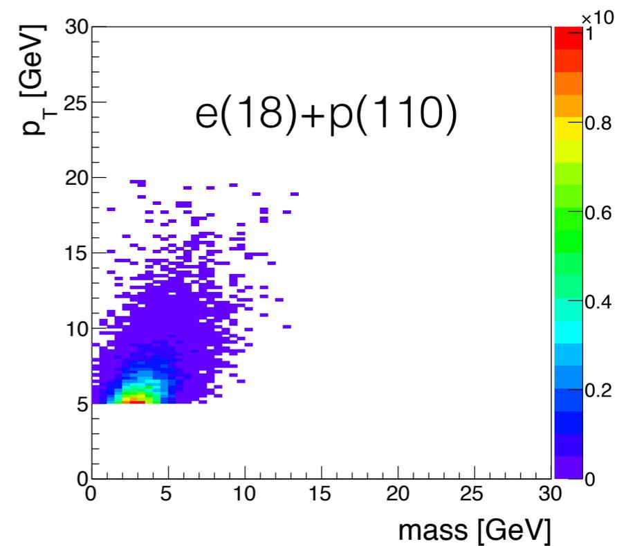
$Q^2 > 10$ ; kT-algorithm;  $R = 1.0$ ; min.  $p_T = 5.0$  GeV/c;  $|\eta| < 4.0$
