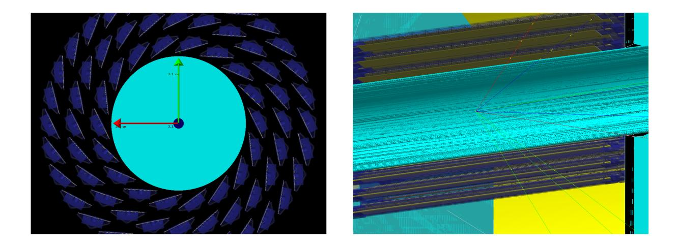
The EIC beam pipe is ~50% larger than the RHIC beam pipe. The MVTX geometry is adjusted to accommodate this pipe. The layout is based on the inner tracker from eRD16/18 from Håkan Wennlöf hwennlof@kth.se.
