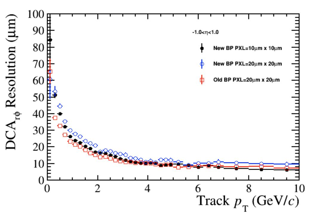
Low pT (=1 GeV/c) resolution about 10  $\mu m$  worse by increasing first layer radius
