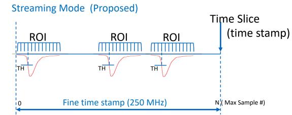
1 Frame = N Clocks (16bits -> up to 262  $\mu$ s for a 4ns clock) (Each FADC can self trigger at the desired Frame Rate)
