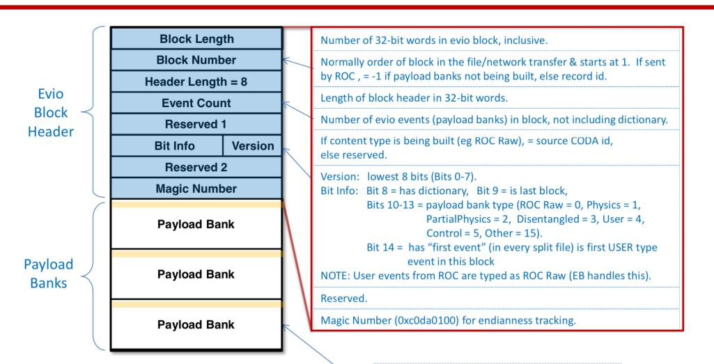
Format used when sending all types of online CODA data over the network. They are in standard evio buffer/file output format with block headers. Each payload bank can be a Physics Event, ROC Raw Record, Control Event, or User event. Note: there may be a block header between any 2 payload banks.
