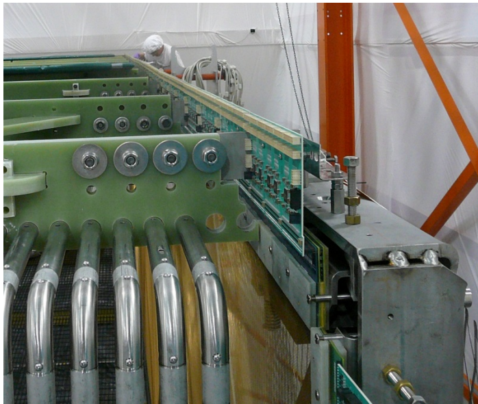
50 cold mother boards (8,256 channels) are installed on MicroBooNE TPC
