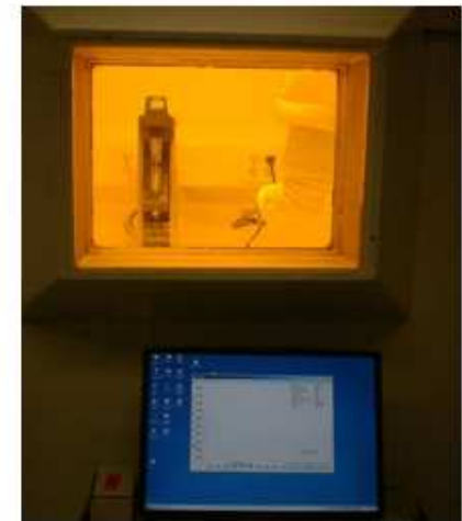
Remotely controlled tensile strength testing
