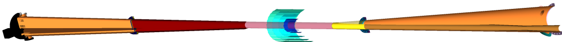
Figure 8.9: GEANT4 model of IR1 Beam Pipe, with Si Vertex Tracker. The electron beam enters horizontally from the right, and exits in the rectangular beam channel to the left. The ion beam enters in the small tube on the lower left, and exits via the large cone on the upper right.
