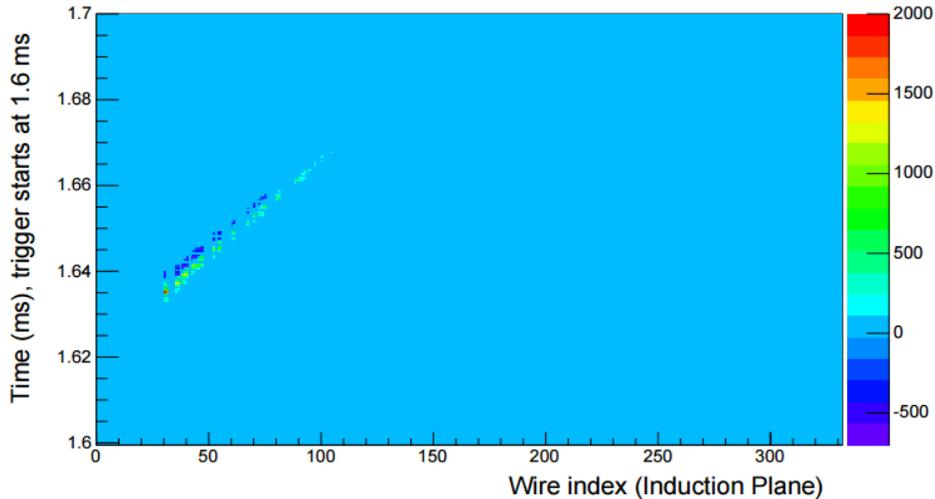
An ionization track from the laser calibration system in Mini-CAPTAIN. The data were collected on August 3, 2015 and were created with a high-intensity UV laser pulse traversing the TPC. The detector was running with one collection plane and one induction plane. The color represents ADC value.
