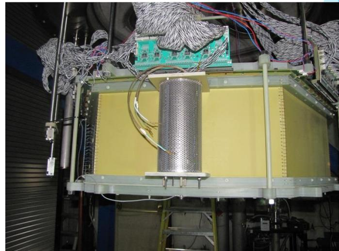
Purity monitoring system has been installed in Mini-CAPTAIN.
